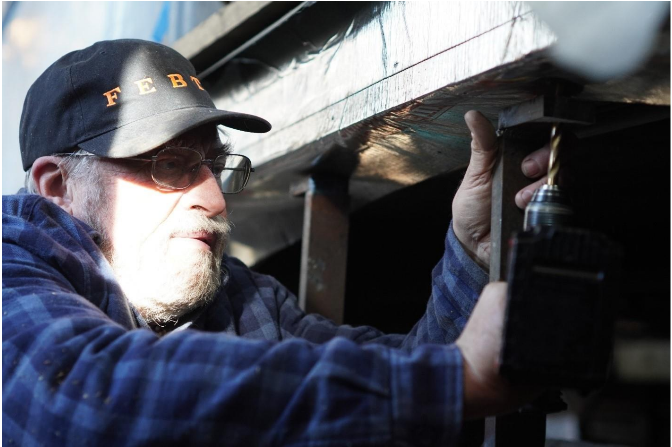
Jim Witmer holds the step stirrup in place below the large baggage door on Combine 14. – Al Gallo photo
