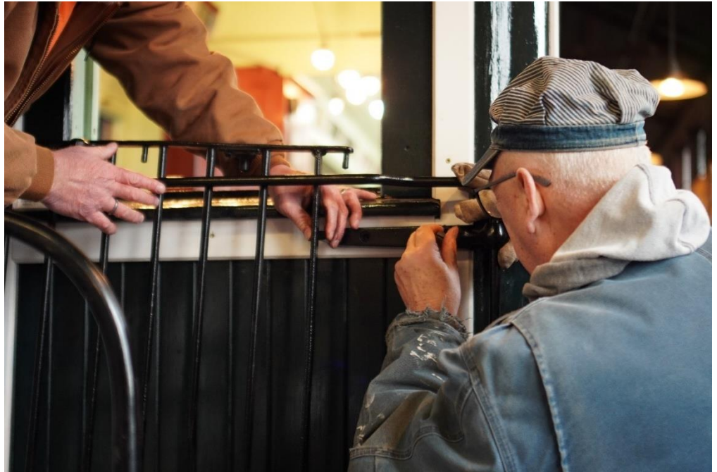
Above: Andy Van Scyoc and Charles Geletzke Jr. install the platform railing on Combine 14. – Al Gallo photo.
