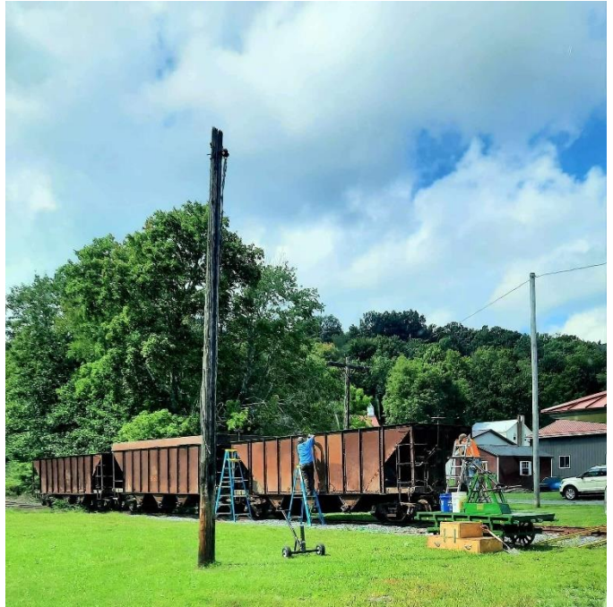
Above: The hopper crew prepping the steel of the car for paint during the September work session. – Dave Camisa photo
