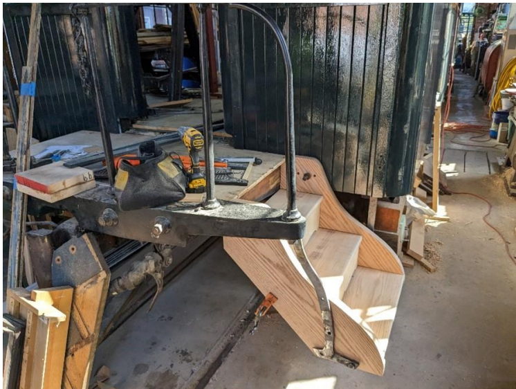
Above: Mark Reese and Charlie Wootten work on fabricating the new platform steps for Combine 14. Left: The first new set of platform steps are trial assembled on Combine 14. – Al Gallo photos
