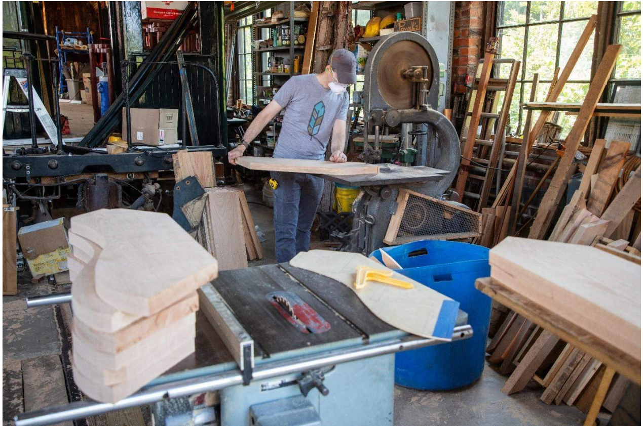
Weston Becker cuts components of the end platforms for Combine 14 during the August work session – Eric Knepp photo
