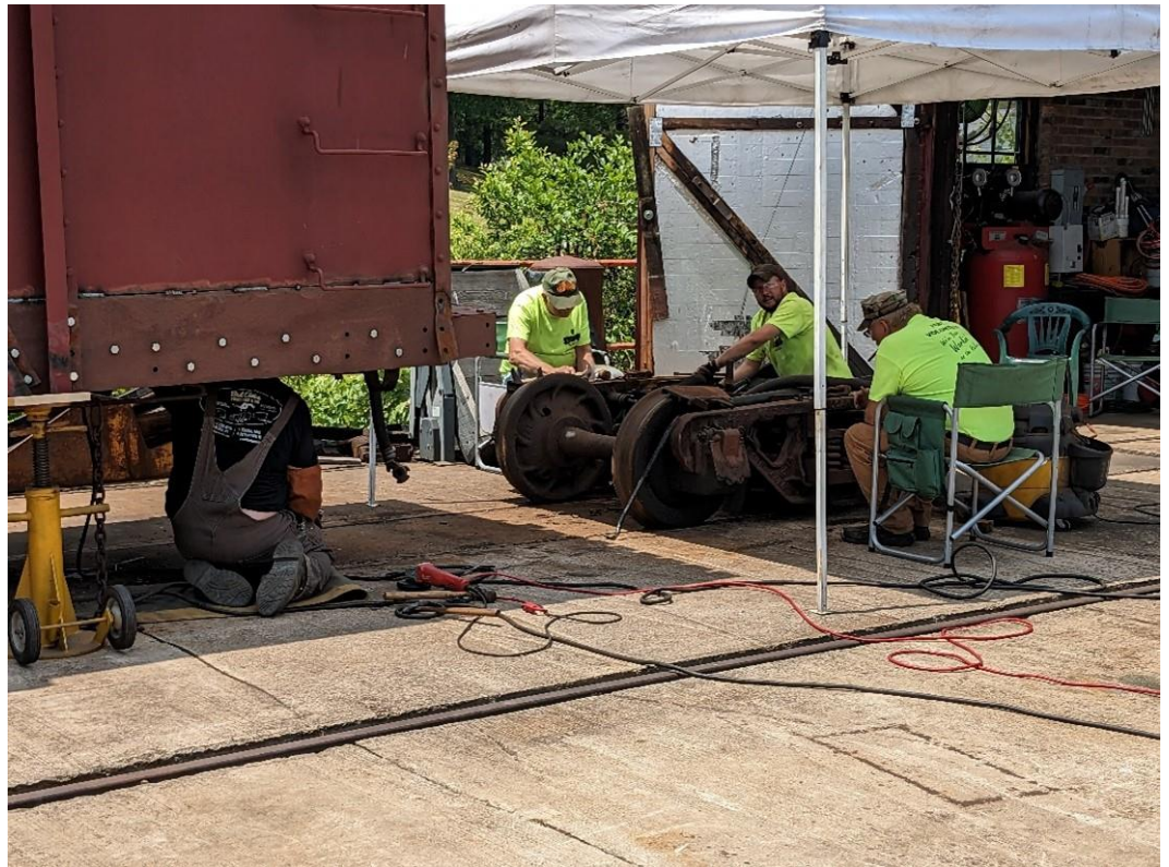
Ben Bilott, Dave Dietz, Alex Cook, and Steve Jacobs perform bolster and truck restoration work on Boxcar 174. – Al Gallo photo
