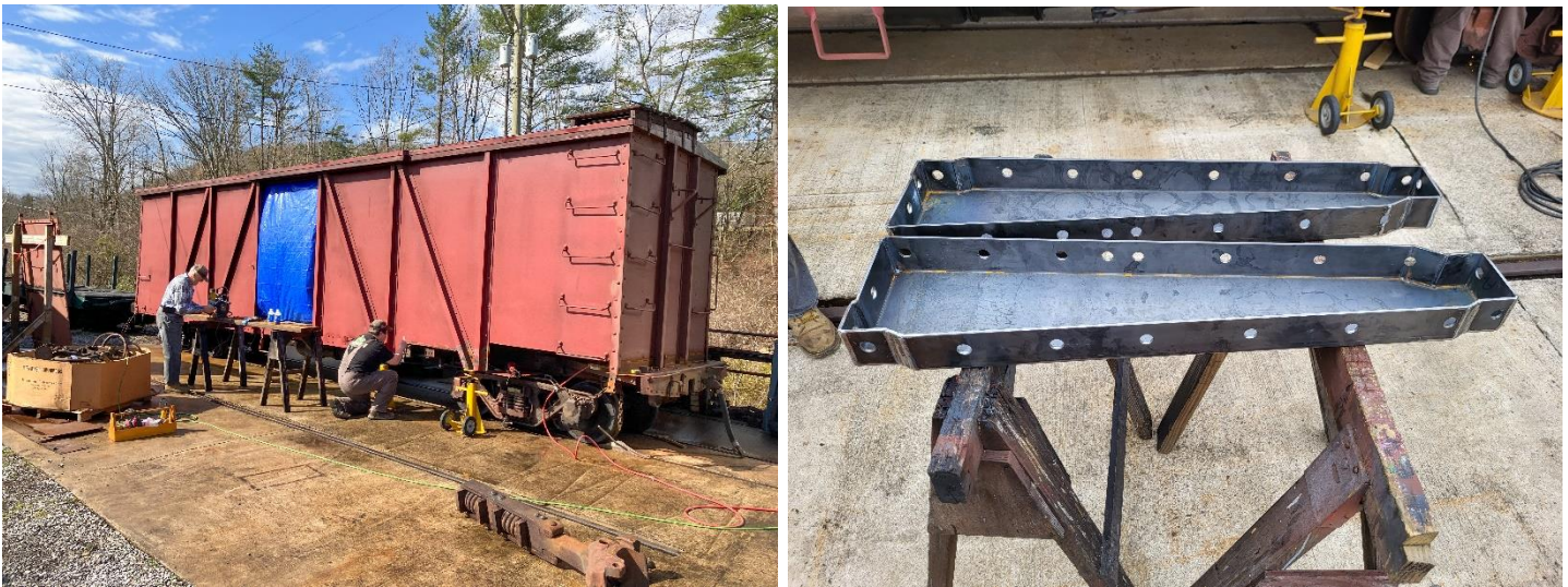
Left: Russell Semen sets up equipment while Ben Bilott makes measurements for Boxcar 174. – Eric Knepp photo Right: New bolster pieces were drawn up by Steve Jacobs, and then fabricated by William and Ben Bilott. – Andy Van Scyoc photo
