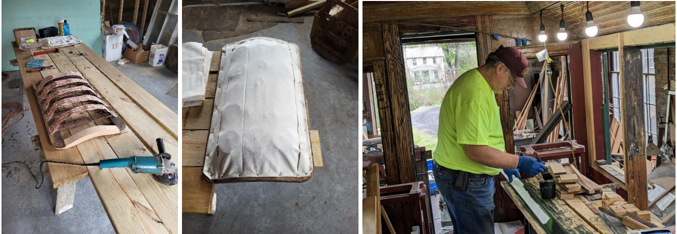
Left: Seat parts have been fabricated to replace any portions that are no longer serviceable. – Andy Van Scyoc photo Center: Once rebuilt, the seats are covered prior to the rattan covering being installed. – Andy Van Scyoc photo Right: Charlie Wootton paints siding for Combine 14 inside the combine, inside the Paint Shop. – Al Gallo photo
